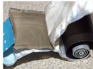
Inside a lithium metal cell
