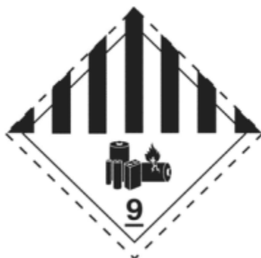
Figure 1. Class 9 Lithium Battery Label
